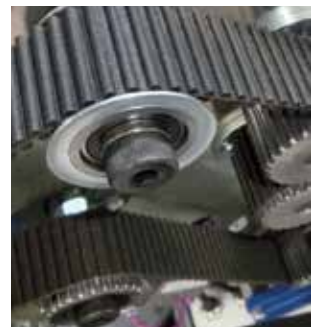
Some of the standard features of the K8RS, from left to right: Palletized feeder, feeder head VacuJet RS, double vacubelt and timing belt drive in the parallel fold.
