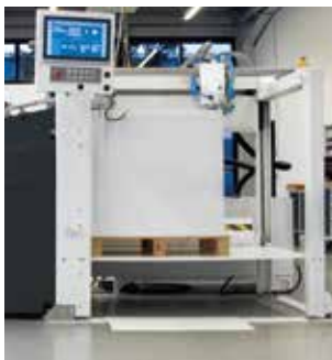
Some of the standard features of the K8RS, from left to right: Palletized feeder, feeder head VacuJet RS, double vacubelt and timing belt drive in the parallel fold.
