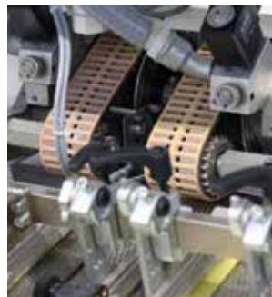
Some of the standard features of the K8RS, from left to right: Palletized feeder, feeder head VacuJet RS, double vacubelt and timing belt drive in the parallel fold.
