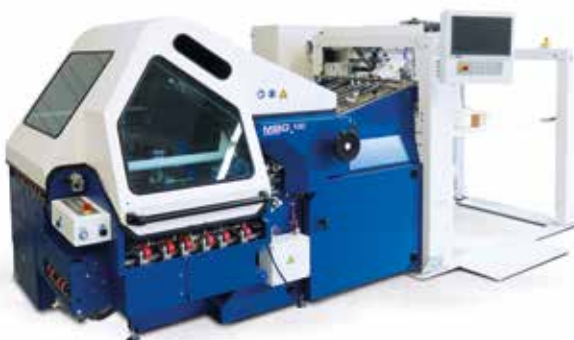
Automated K80 with palletized feeder.
