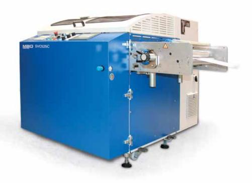
The SVC sheeter is variable and fully electronically adjustable in terms of format and chip-out size. Due to its solid industrial construction, the SVC series is designed for the highest customer requirements and maximum running performance – even in continuous operation. However, due to the high level of automation and minimum set-up
